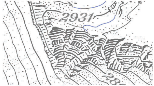
Figure 20. The arrangement of strokes parallel to contour lines compensates for omitted intermediate contour lines at 1 : 25 000
