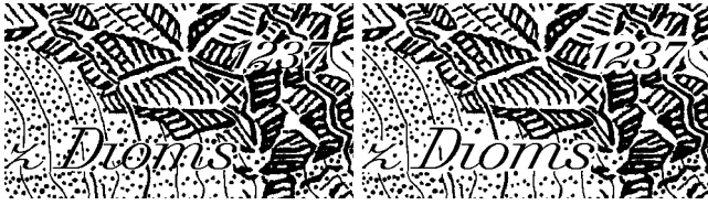
Figure 10. Masking of scree and rock drawing to improve type readability (enlarged) (Spiess et al. , 2002)
