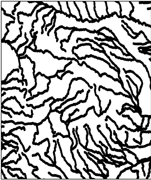
Fig. 8. Buffered drainage network: dark areas indicate valley bottoms where lower quartile filter is applied.
