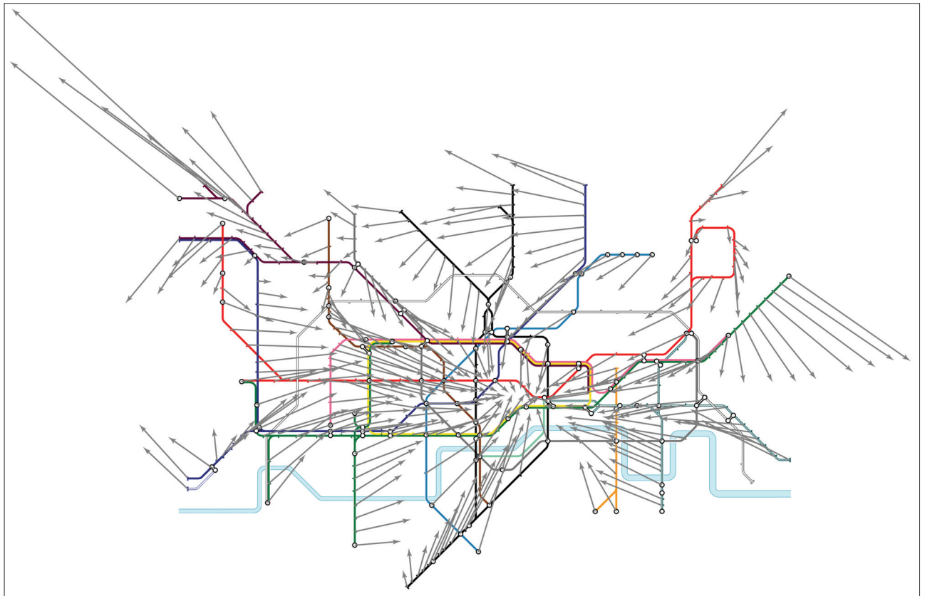
Figure 3 Displacement vectors. Arrows point at the correct geographic location of each station.
