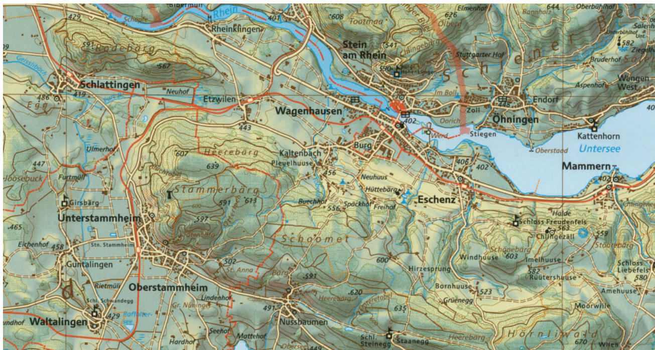
Figure 15. Computer-generated colours derived from a hand-drawn grey relief shading using colour reference points and a look-up table
